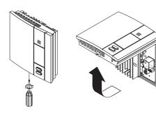
Make the connections using solderless connectors for copper wires. The thermostat wires are non-polarized; this means either wire can be connected to either terminal.
