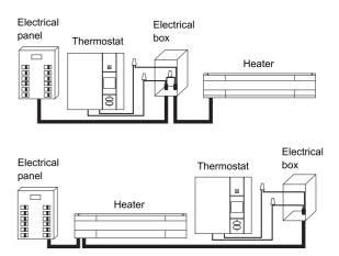
**WARNING**: This thermostat has tinned copper wires for line and load connections. Special CO/ALR solderless connectors must be used when connecting with aluminium conductors.
