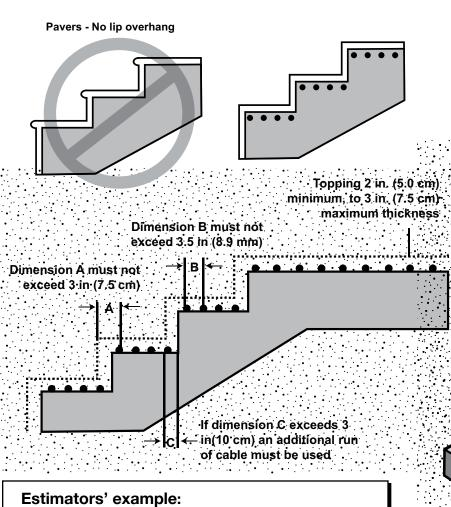
Stair treads have to be 11-12" deep. Landing =  $4' \times 6' = 24 \text{ sq.ft } X = 96 \text{ FT}$ 3 steps (12" x 6' each) ... we want 4 passes of cable per tread. Subtract 3" from each side (making room for hand rail posts) 5.5' X 4 = 22 FT plus 3 FT = 25 FT per tread 3 FT is the amount needed for curves and tread riser.
