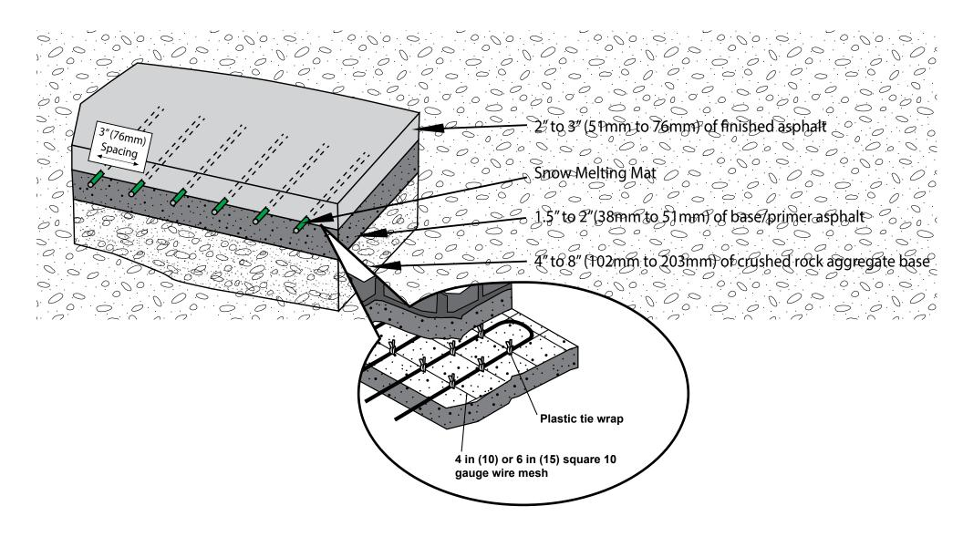
Note: Cables may be tied to reinforcement type mesh and then the mesh should be staked down to the base/primer pour.
