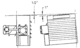
Maximum tilt allowed during operation (applicable front to back and side to side in either direction). Heater must be permanently mounted.
