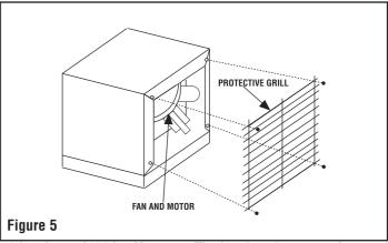
10 kw through 30 kw Heaters: The heating element surface and fan motor area are accessible by removing the left or right side panel of heater. To do this, open the hinged control box cover, and then remove the two screws that hold the bottom of the side panel. Lift out that end of the side panel and then pull down for removal. After servicing the unit, reverse the unit, reverse this procedure to replace the side panel.
