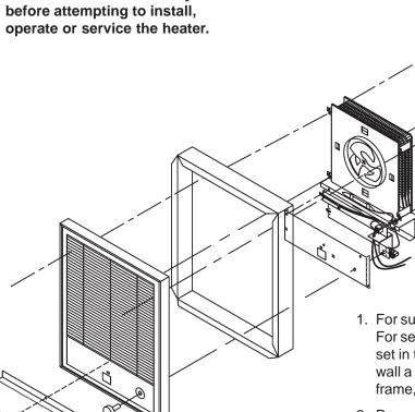
1. For surface mounting attach 3450/AFC box to wall. For semi-recessed mounting 3450AFC box should be set in the wall so the flange is out from the finished wall a distance equal to the frame depth (1" for a 1" frame, 2" for a 2" frame).
