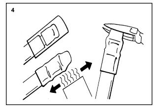
Heat-shrink 3/4" x 4" heat-shrink tube in place with  $^3/\epsilon$ " over end of smaller heat-shrink tube. Remove heat, resqueeze at end of smaller heat-shrink tube, then squeeze at end of outer heat-shrink tube. Hold for 10 to 15 seconds.
