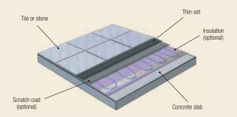
**Recommended cable spacing:** *Two-inches* when installed over concrete slab; three-inches when installed over insulated concrete slab.
