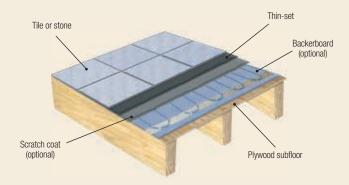
**Recommended cable spacing:** *Three-inches when installed over wood sub-floor.*
