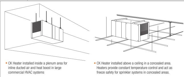
• CK Model for heating large HVAC air intake systems. Provides pre-heating for controlled HVAC multiple floor supply systems
