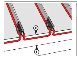
The architectural conditions below the drip line of each metal roof (D) varies greatly. The facia (F) may be wood or clad in sheet metal. There may be drip edge flashing or a gutter, or both, for example. The treatment of the horizontal cable areas will therefore be different from job to job. Some installers prefer to use a standard IDP-113 roof clip to secure this area as illustrated on page one (D).
