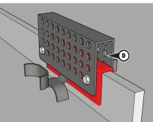
As noted, there may be a gap (D) between the top of the GVG clip and the standing seam. This will not affect the performance of the clip. During installation, the GVG clip should be pushed down until the cradles touch the main surface of the metal roof or the clip sits on top of the seam.
