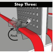
Step Three: After fastening the clip, lay the heat cable into the cradle (C) and use your fingers to pinch the top half of the cradle down onto the cable. A pliers may also be used for the pinching process.
