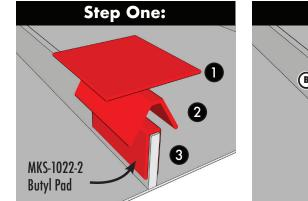
Step One: Peel the backing off both sides of a butyl pad (MKS-1022-2) and fold it over the standing seam at the desired clip location. Clean the area first with a rag and common isopropyl alcohol (rubbing alcohol) to ensure a good bond between the butyl and the metal. For best results, keep the butyl pads warm before installation.
