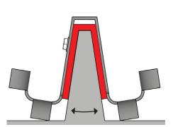
The GVG clip can be modified on site to fit a variety of circumstances. Here, the legs of the clip were spread slightly to accommodate a triangular shaped standing seam.
