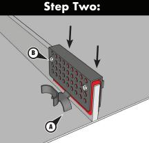
Step Two: Set the clip onto the seam until it either rests on top of the seam OR the cradles are touching the roof (A). Using a drill and a 5/16'' hex head driver bit, fasten the clip to the seam using two provided self-tapping sheet metal screws. Install screws near the top of the seam (B) to reduce likelihood of water ingress into the roof system. Do NOT over tighten screws as they will strip the holes.
