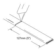
2. Lightly cut overjacket up the center between first cut mark and the cable end. Bend cable to break overjacket.
