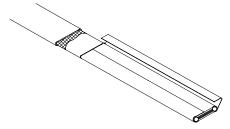
11. Shave the core material from the outside of each bus wire.
