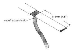
8. Lightly cut around heater jacket 4" (102mm) from the end. Bend cable to break outer jacket.
