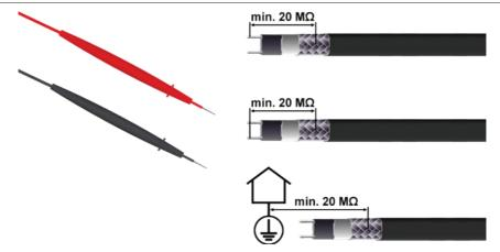
**NOTICE:** The heating circuit must not be grounded.
