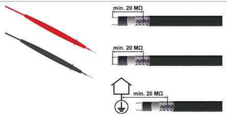
**NOTICE:** The heating circuit must not be grounded.
