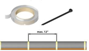
**NOTICE:** In order to ensure good heat transmission the trace heater must have a flat, flush fit over the whole length. If necessary, reduce the distances between the fixing points.
