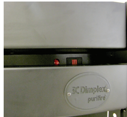
Exterior View of Voltage Selector Switch and Over Temperature Light
