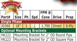
OSHA requires this fan to be mounted a minimum of 7' above the floor.
