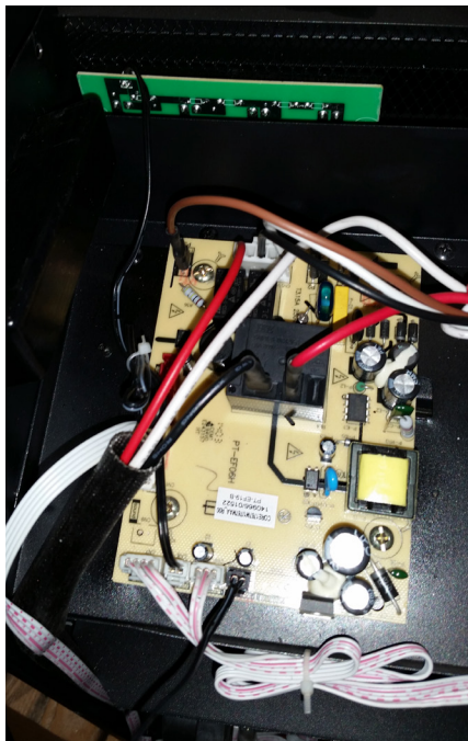
Control Board and Switch Board
